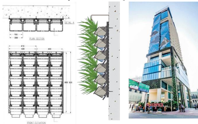
Figure 3: Living wall system details in the Sri Lankan market and Mövenpick hotel (Wall Span, 2017)
